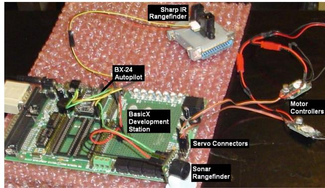
Figure 9. Autopilot breadboard with sensors.
