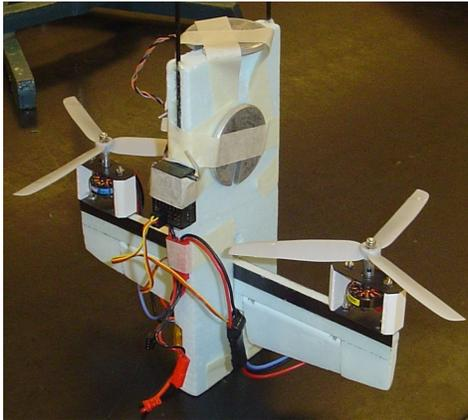
*Figure 4. Gondola with lift fans and vanes.*
