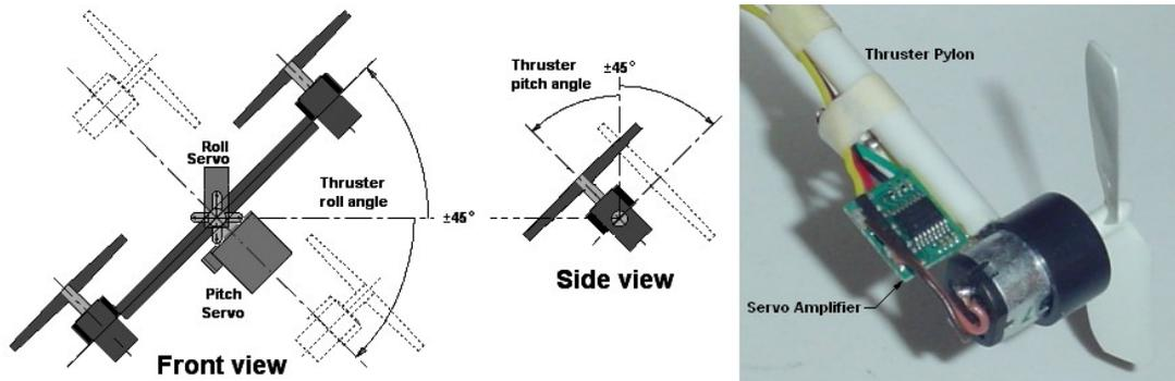
Figure 3. Propulsion thrust vector control.
