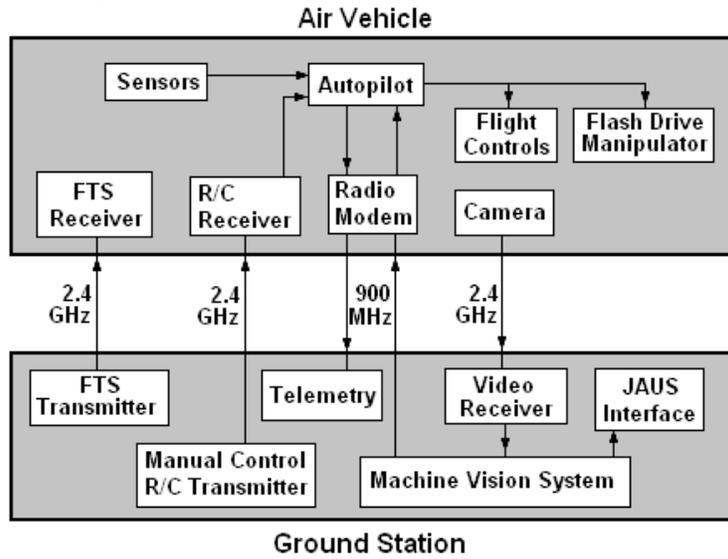
Figure 1. Overall system architecture.
