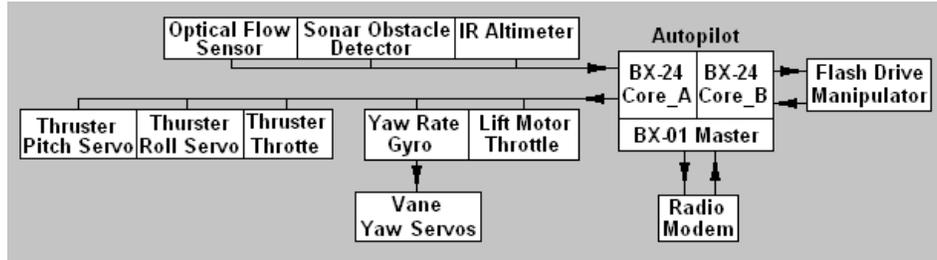
Figure 5. Control system architecture.
