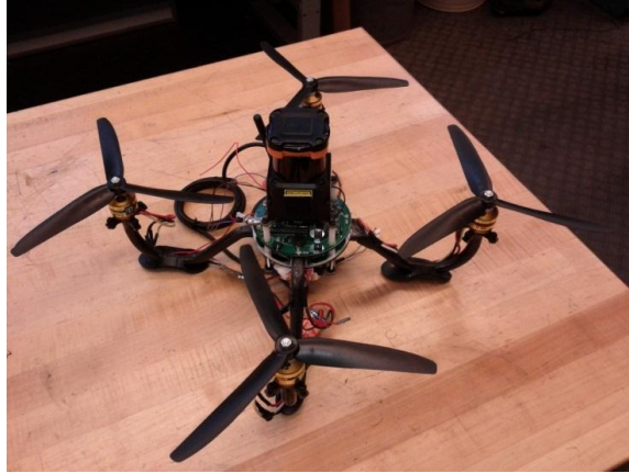
Figure 2: An overhead shot of the MAAV quadrotor fully assembled
