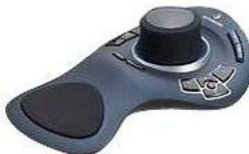
Figure 9: 3DConnexion SpaceExplorer used for manual flight during the testing phase.
