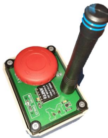
Figure 5: The custom designed and fabricated kill switch that broadcasts over its own frequency
