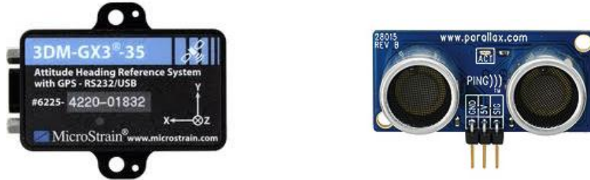
Figure 6: The Microstrain 3DM-GX3-25 (left) Ping ultrasonic range finder (right). These two sensors are mounted on the vehicle to monitor roll, pitch, yaw, and height.
