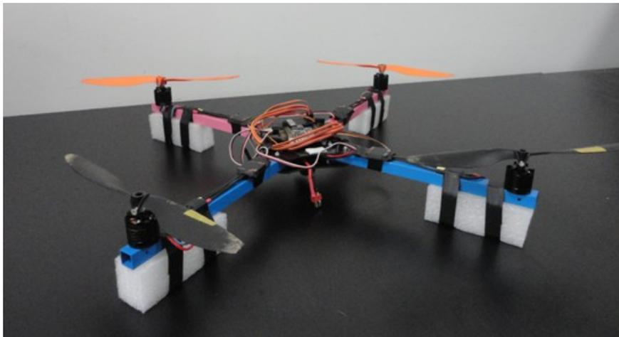
Figure 1: The Quadrotor Platform of the UAV System
