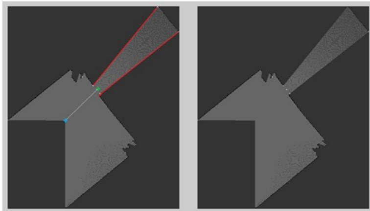
Figure 6: The Path Planning Result in a Corridor Environment
