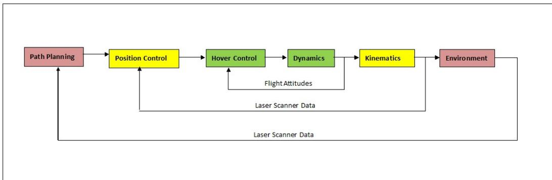
Figure 3: The Software Structure Diagram
