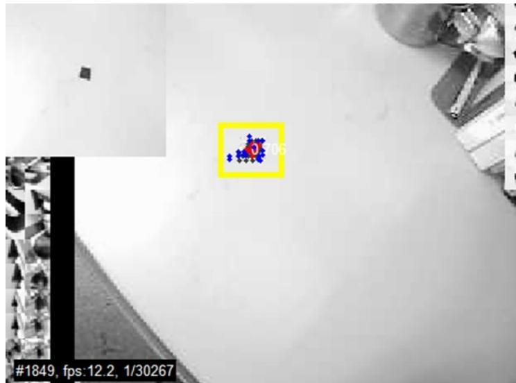
Figure 4: Using the TLD Method to Track a Chip
