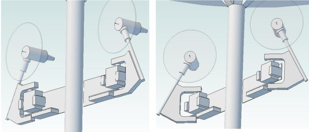
*Figure 3. Propulsion thrust vector control. At left, thruster is centered. At right, thruster is deflected 45°.*
