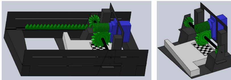
*Figure 6. Flash drive retrieval mechanism, scoop on right. The checkerboard pattern denotes a groove that holds the decoy.*
