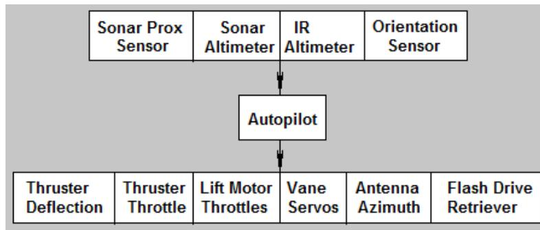
Figure 5. Control system architecture.
