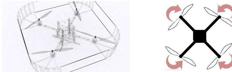
(a) AscTec Pelican Platform (b) Quadrotor Propulsion and Lift System
