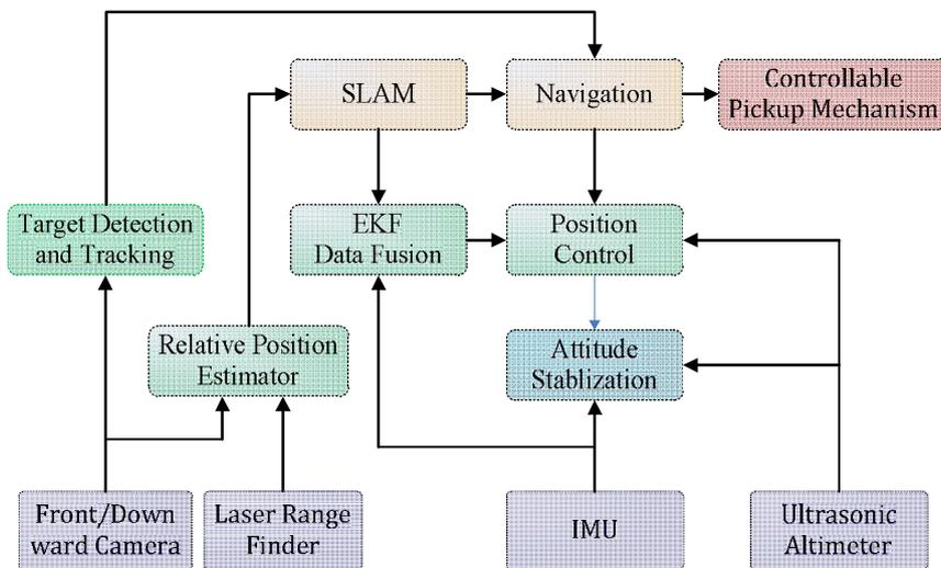
Figure 4. The control system architecture.
