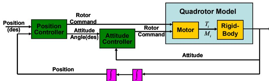
Figure 3. The inner-outer control schematic of the THRONE quadrotor
