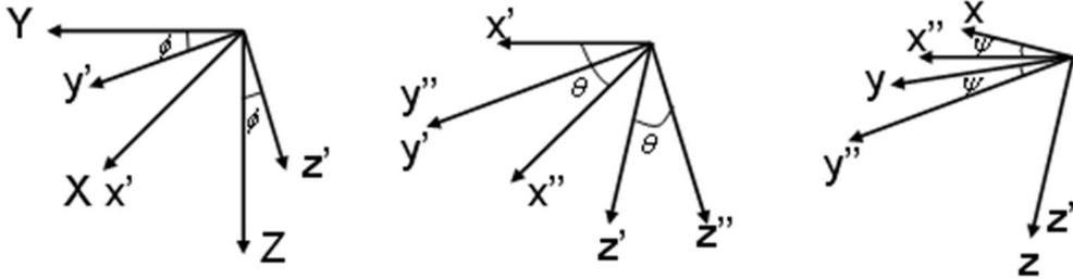
Figure 8. Sketches of pitch roll and yaw.
