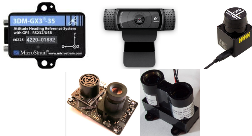
Figure 3: From left to right and top to bottom, The Microstrain 3DM-GX3-25, Logitech C920 Webcam, Hokuyo URG-04LG-UG01 Laser Rangefinder, PX4 Optical Flow Sensor, and Pulsed Light Lidar-Lite Laser Module
