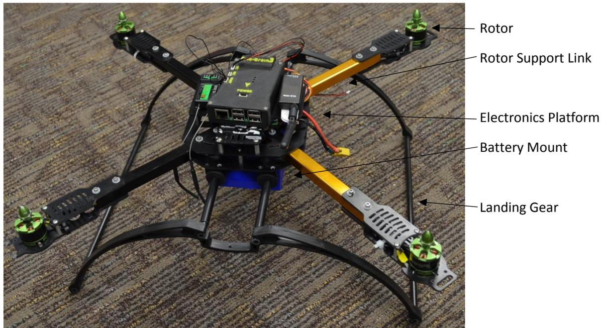
*Figure 2. Chassis of UAV with key electromechanical components labeled.*
