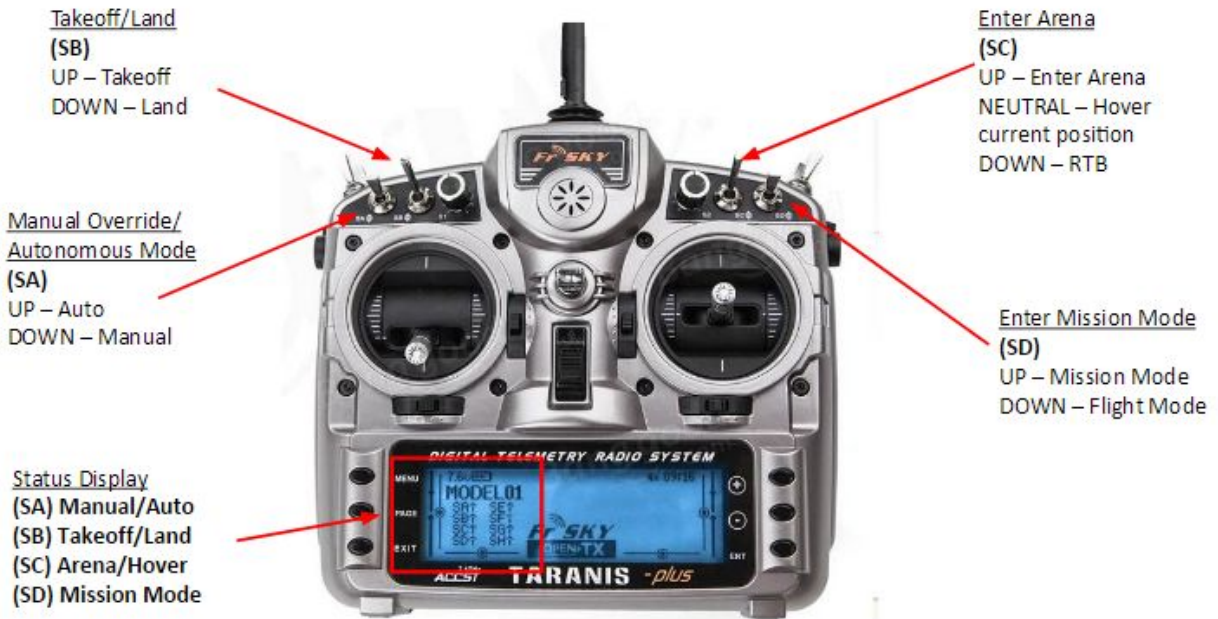
Figure 4. RF Control Station
