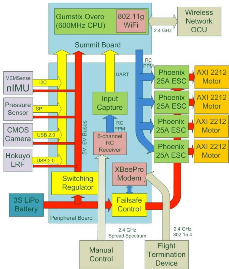
Figure 1. Overall System Architecture
