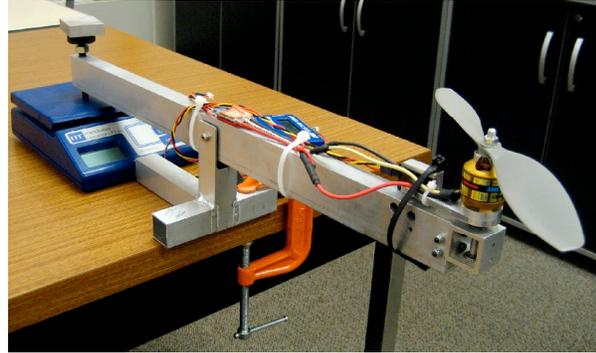
*Figure 4. Motor Test Platform*
