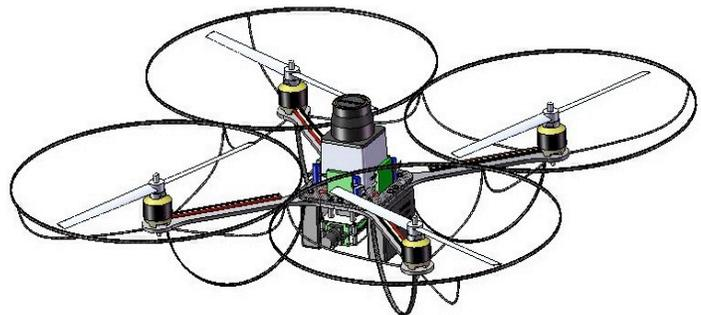
*Figure 2. CAD Model of SERV*
