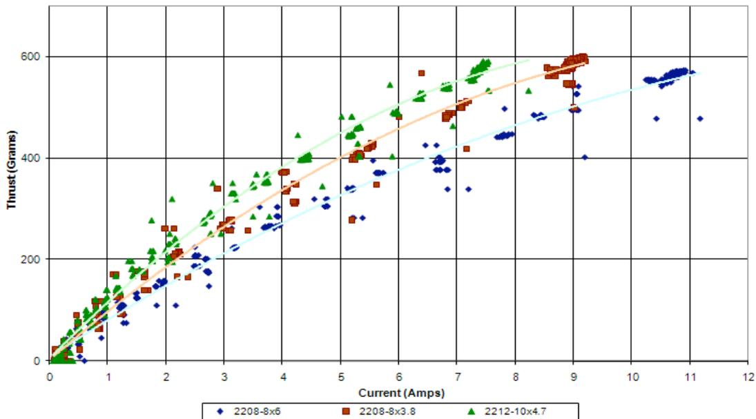
*Figure 5. Thrust vs. Current Plot*
