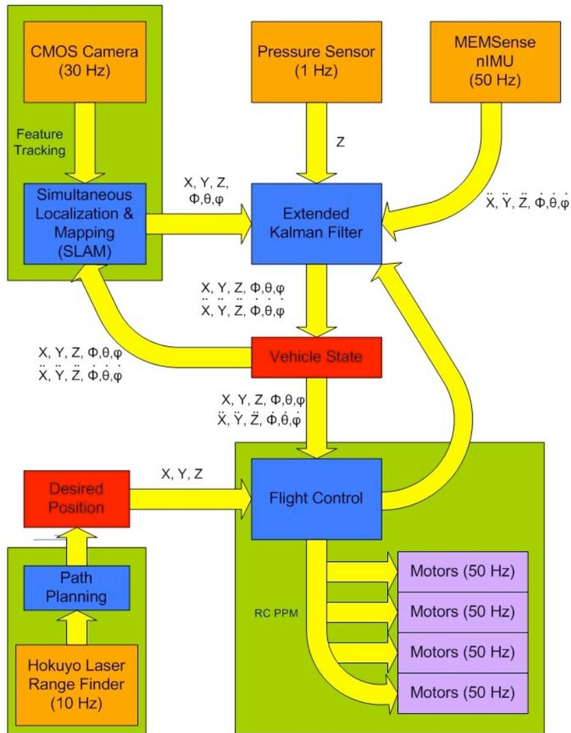
Figure 3. Control System Architecture
