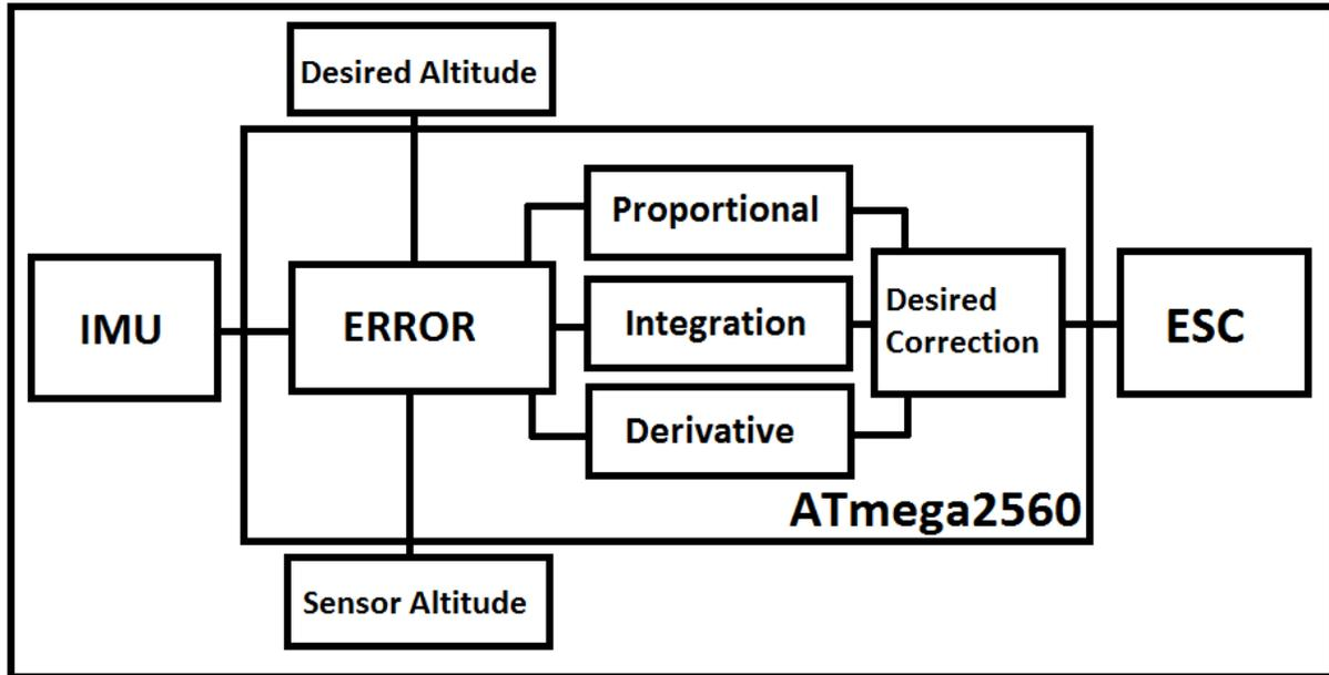
Figure 2. Simplified PID Logic Flow Diagram
