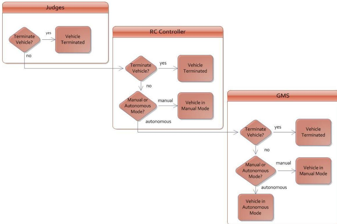
*Figure 4: Man/Machine Interface Command Hierarchy*
