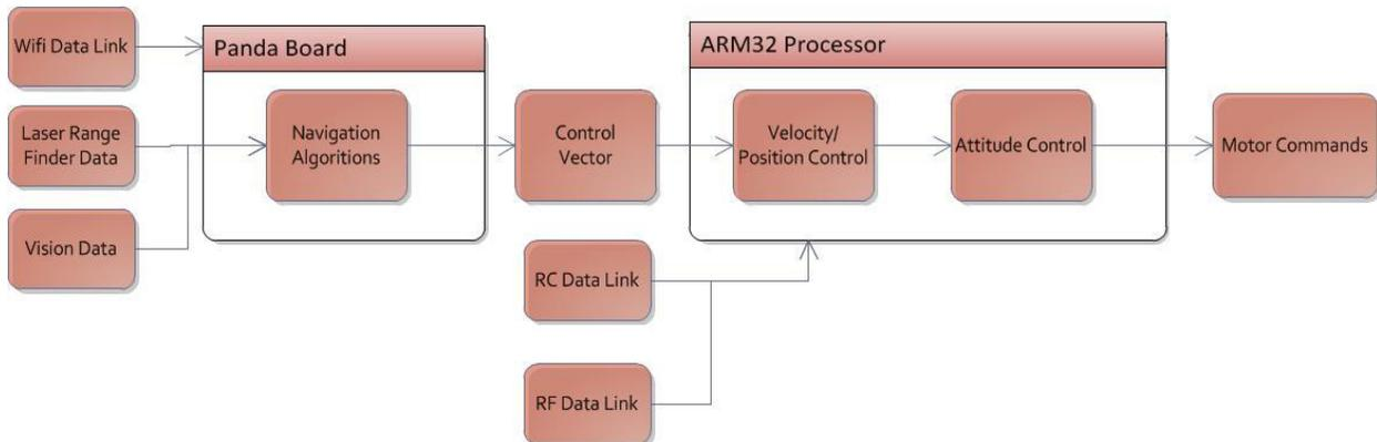
*Figure 3: Control System Architecture*
