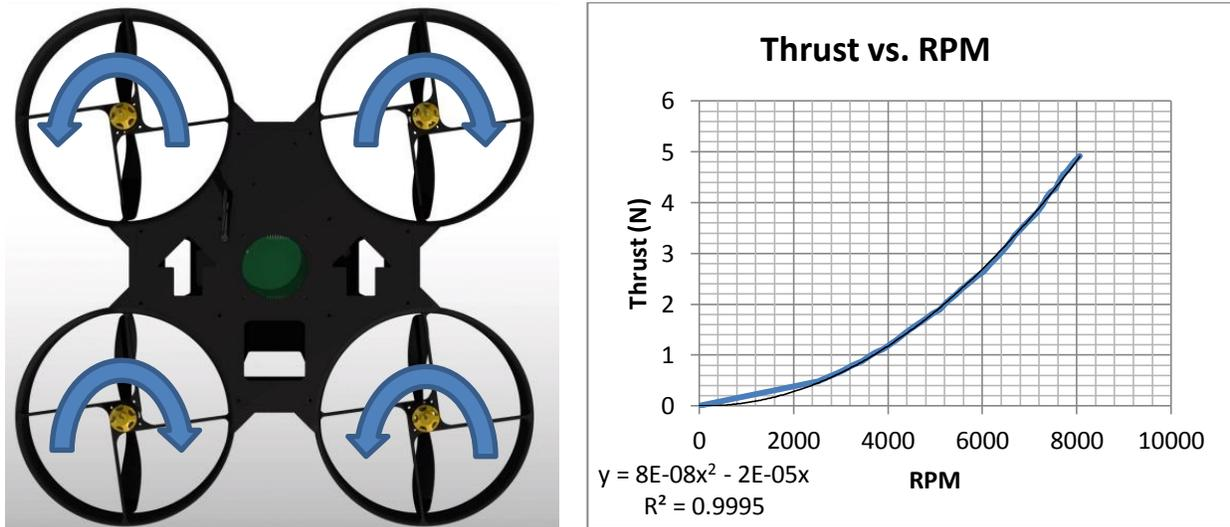
Figure 2: a) Rotor configuration b) Thrust vs. RPM curve for motor/propeller combo
