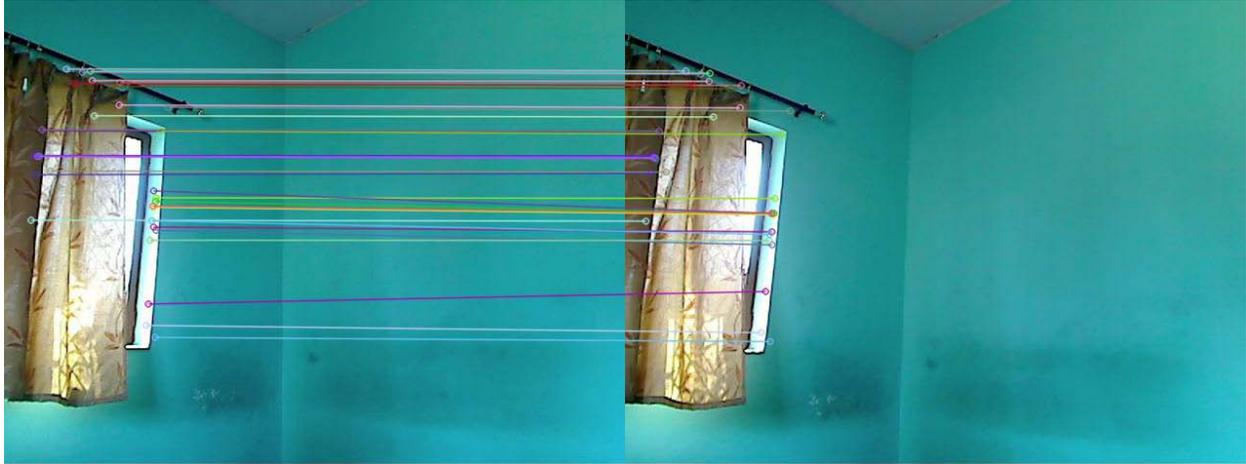
**Correspondences between the SURF keypoints detected in both images**
