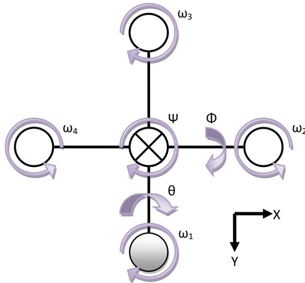
Figure 1: Quadrotor Body Diagram
