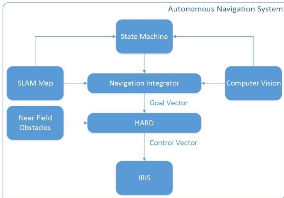
*Figure 3: Autonomous Navigation System*
