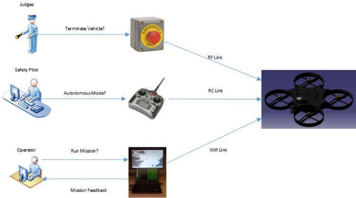
**Figure 5: Man/Machine Interface Hierarchy**
