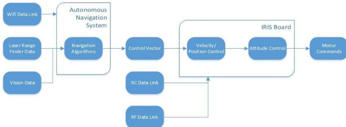
Figure 4: Control System Architecture
