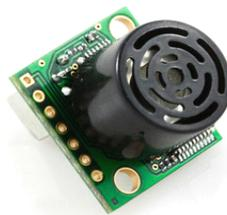
*Figure 3 Maxbotix ultrasonic height sensors*
