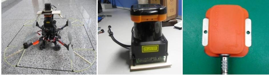
Figure 5. Our quadrotor platform (left), UTM-30LX laser range finder (middle) and XSens IMU (right).
