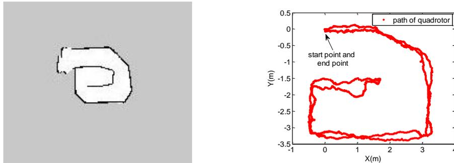
Figure 6. Map of Tsinghua experimental site (left) obtained in real time using our algorithm, and the trajectory of our quadrotor (right) after closing the major loop.
