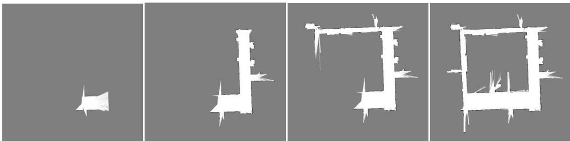
Figure 7. Incremental mapping of New Main Building of Beihang University. The left image shows the initial map and the right image shows the resulting map.
