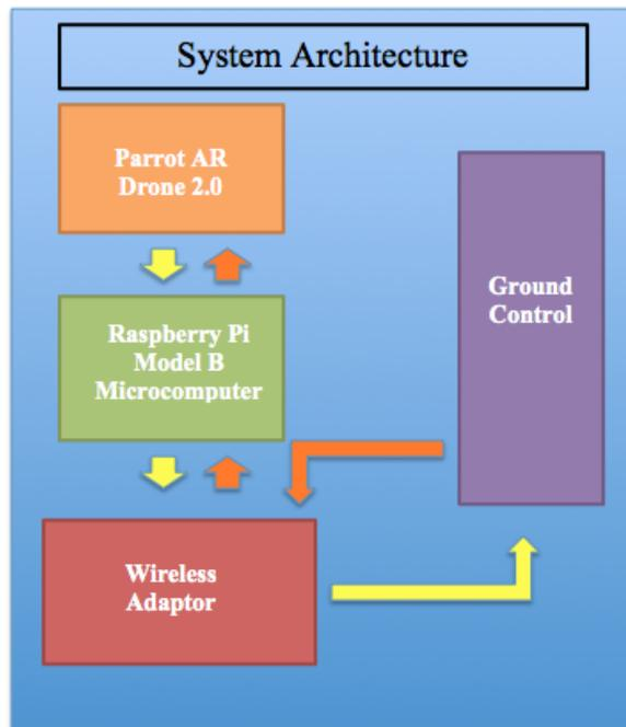
Figure 2, System Architecture of APUS
