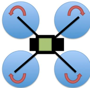
*Figure 1, Motor Configuration of the Vehicle*
