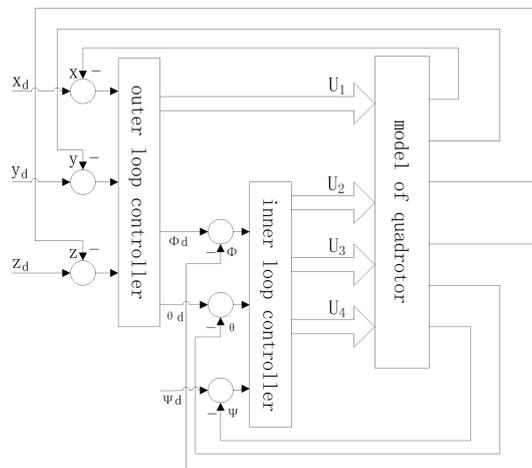
Fig2.4 Structure of the double loop PID control system
