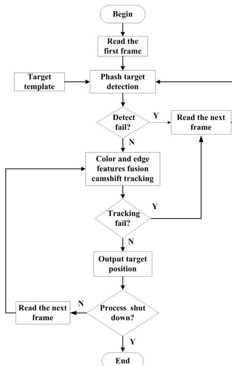
Fig2.6 Ground target tracking algorithm
