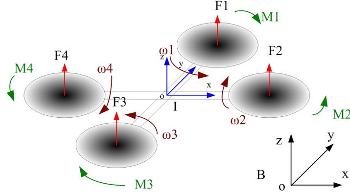
fig 5.2 structure of the vehicle
