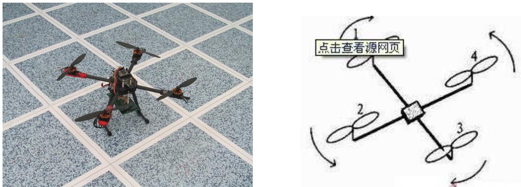
Figure 2:quadrotor and the propeller action
