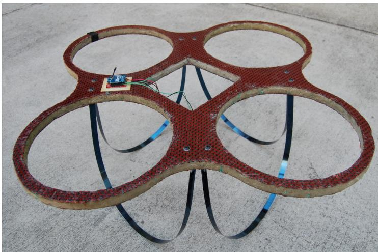
*Figure 5: Propeller guard with landing gear mounted.*
