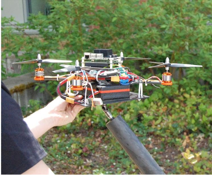
*Figure 9: Quadrotor on test mount.*
