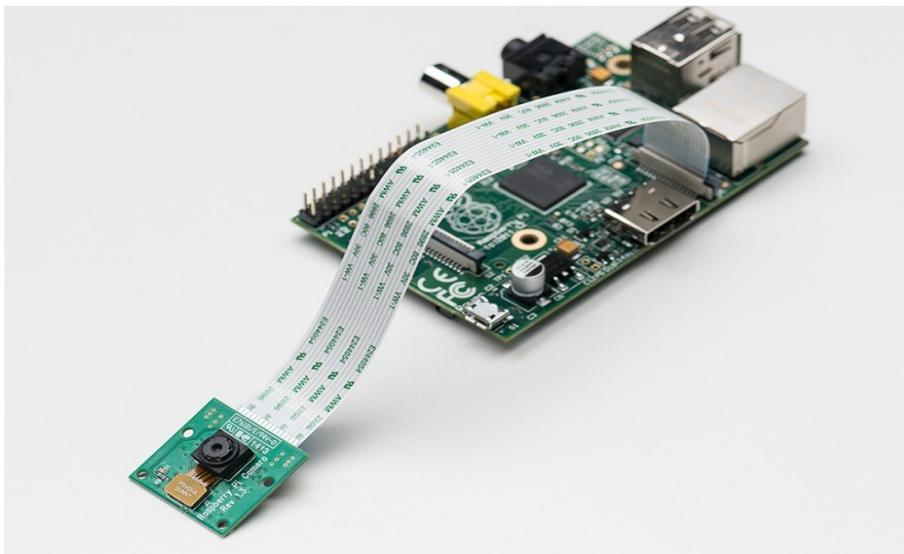
*Figure 6. Raspberry Pi with camera.*
