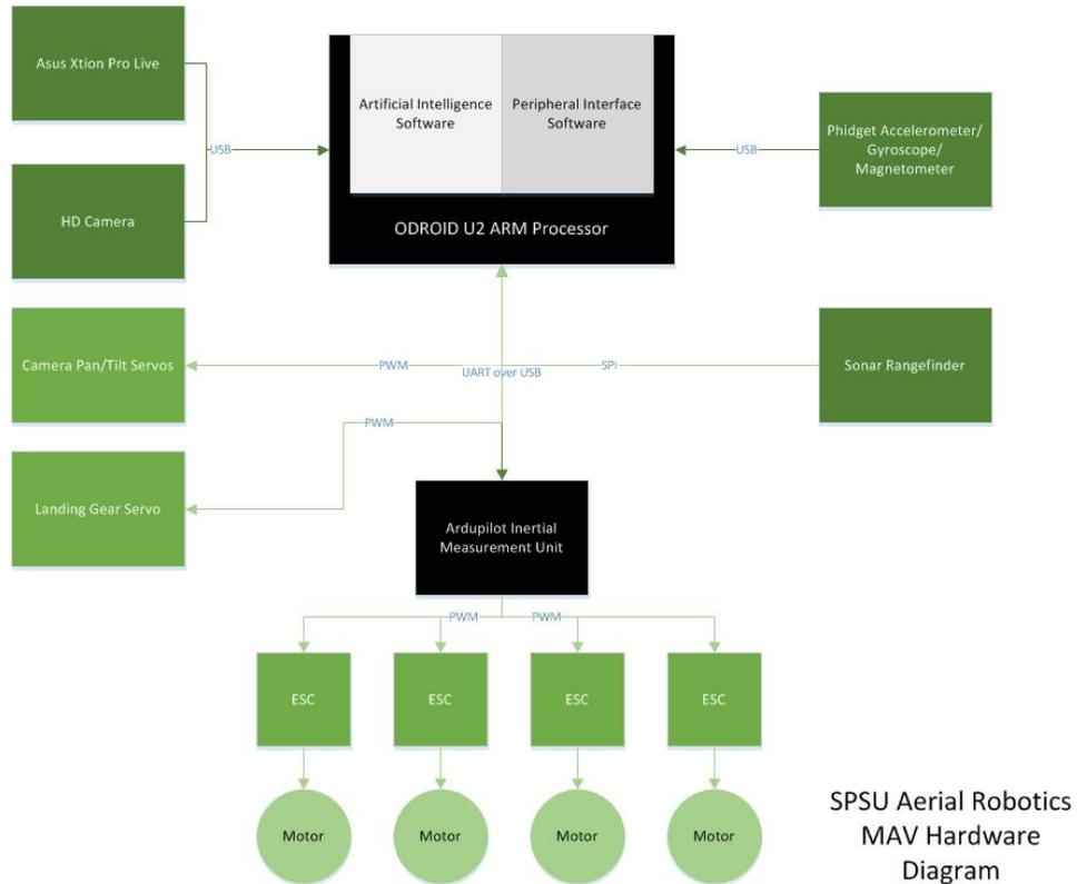
Figure 1.0 – SPSU Aerial Robotics MAV Hardware Diagram
