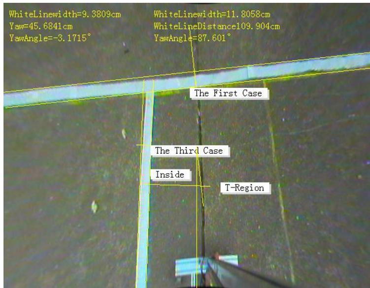
Figure 7. Detect Intersection Lines
