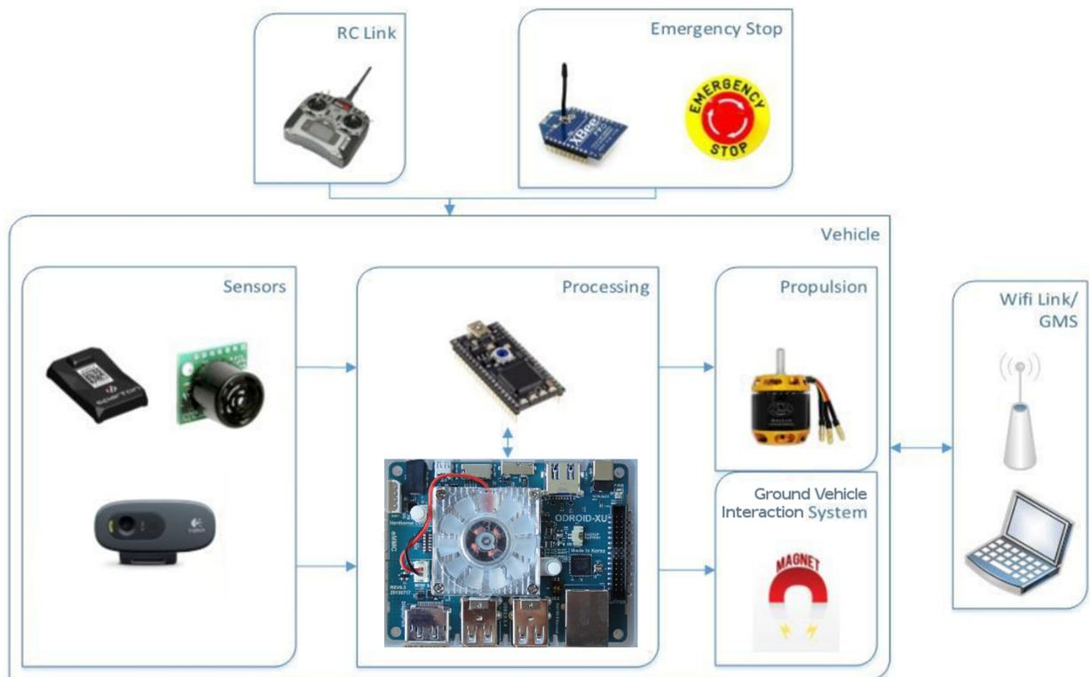
**Figure 1: ERAU RAVEN II System Architecture**
