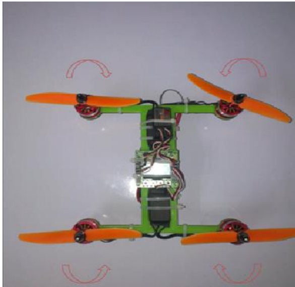
(a) Quad rotor Propulsion and lift system
