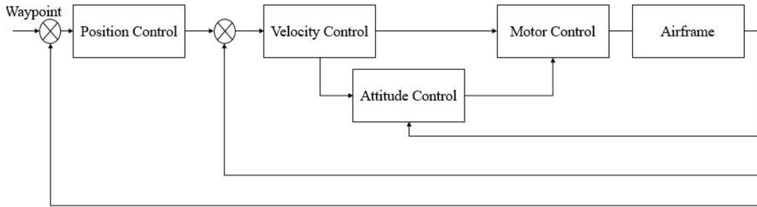
Figure 2: Structure of Control System
