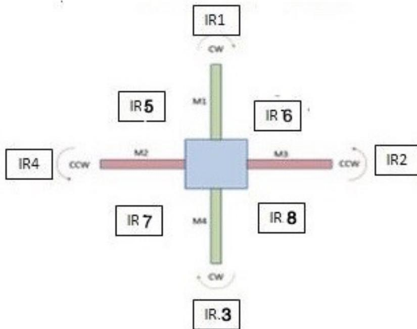
**Figure 7. Placement of IR sensor on the quadcopter.**
