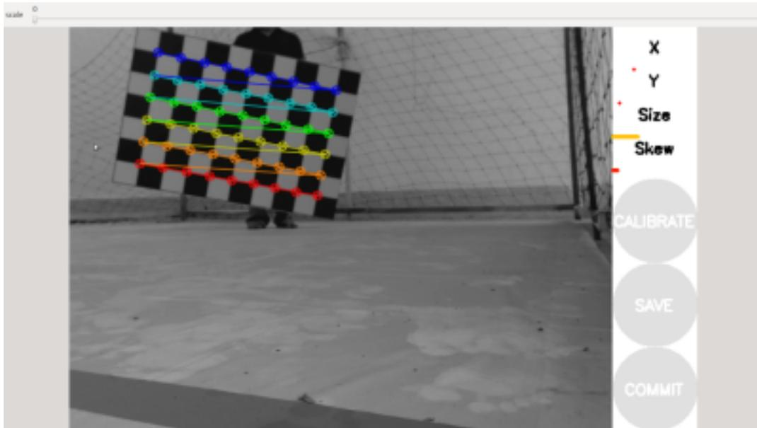
Figure 10. Left and right Camera Calibration using 9\*6 checkerboard
