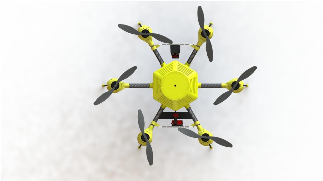
Figure 2: A render of the top view of the multirotor airframe.
