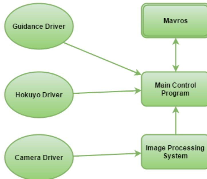
Figure 3: Sensor network diagram.
