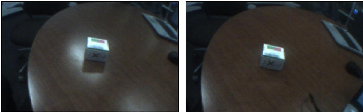
*Figure 7. Glare reduction comparison: without polarizer vs with*
