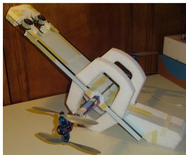
*Figure 9. Vehicle in inverted takeoff orientation.*
