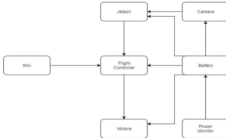
*Figure 1. Overall System Architecture*
