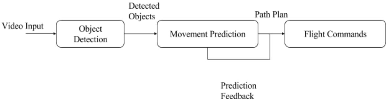
Figure 3. Object Tracking Software Design
