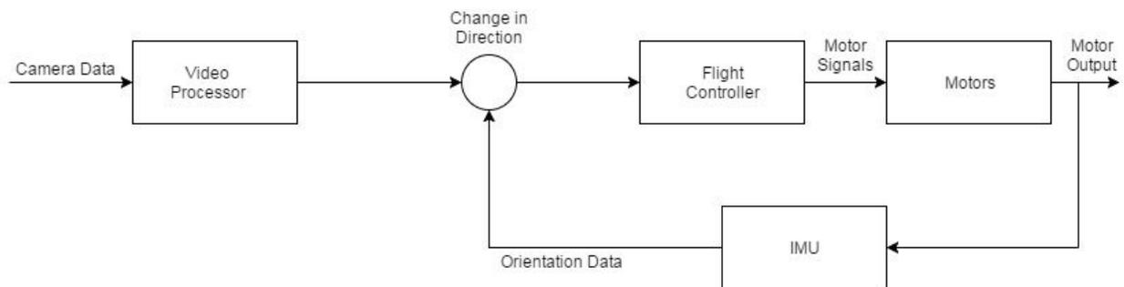
Figure 3. Quadcopter Control Loop
