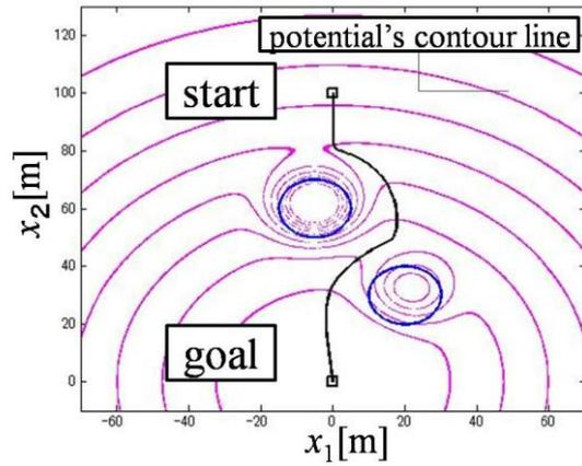
Figure 12: Artificial potential field approach
