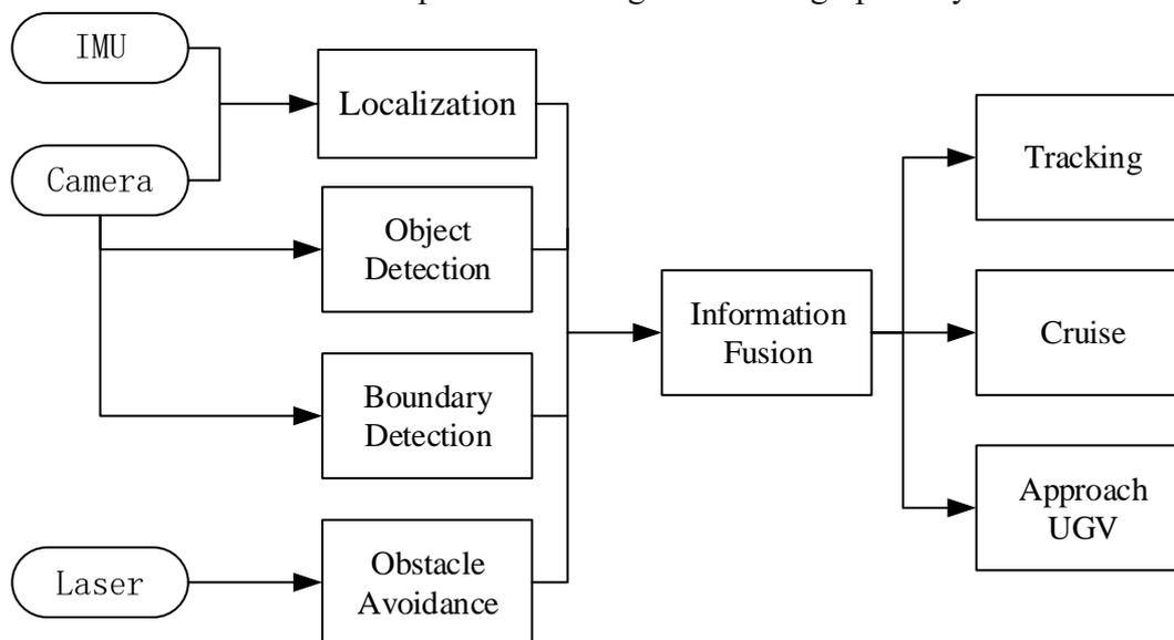
Figure 7: AGV system structure
