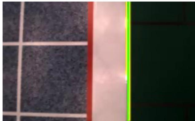
Figure 11: Boundary detection from down-sight camera (boundary is labeled by green line)
