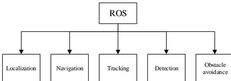
Figure 6: Modules of software in UAV system
